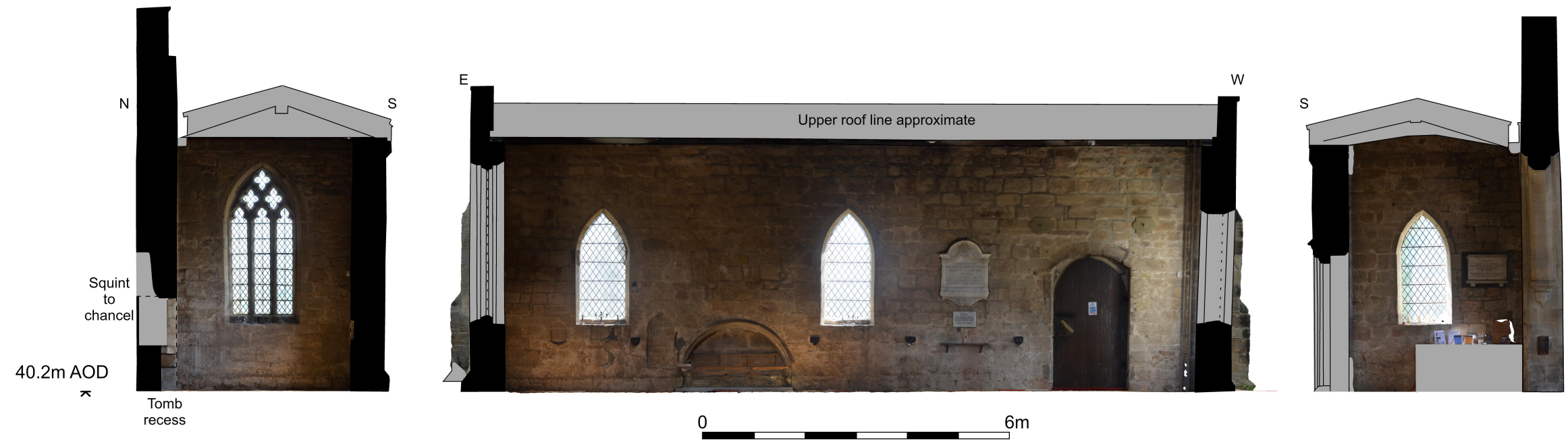
Internal elevations of south aisle. L-R: west face of east wall looking east, showing squint cutting through the adjacent nave wall; north face of south wall looking south; and east face of west wall looking west.
