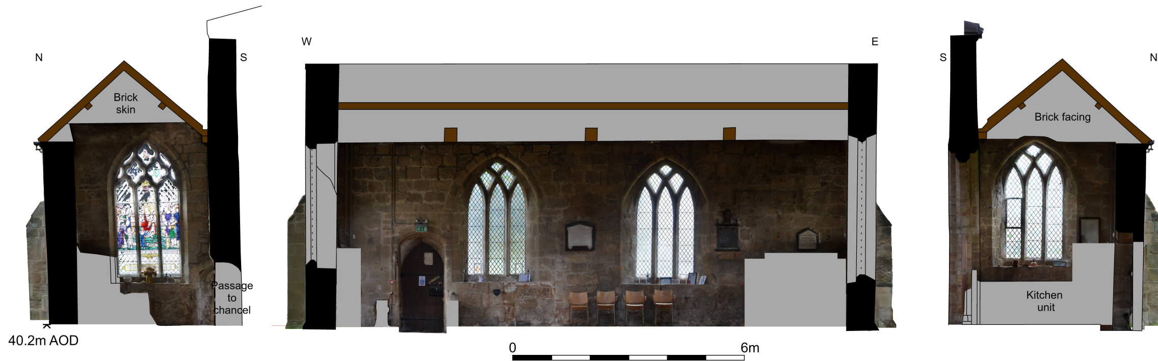
Interior elevations of north aisle, West face of east wall looking east; south face of north wall looking north; and east face of west wall looking west.
