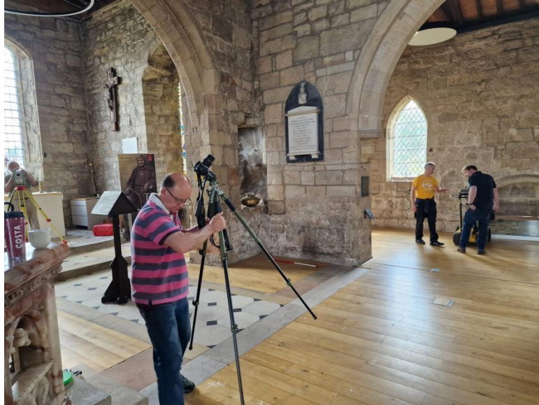
Photograph 4_4: Volunteer moving camera on tripod to take overlapping photographs of the church interior for photogrammetric survey
