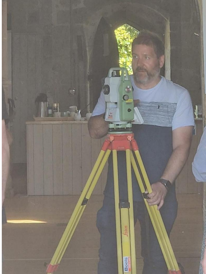
Photograph 4_2: Leica TS07 EDM Total Station being set up in the entrance to St Wilfrid's from GPS control points outside.
