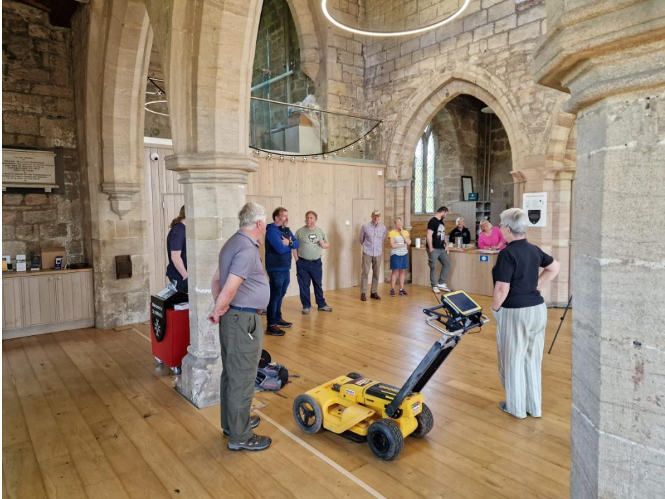
Photograph 4_1: Volunteers being briefed on Ground Penetrating Radar survey techniques. The Leica DS2000 GPR is in the foreground.
