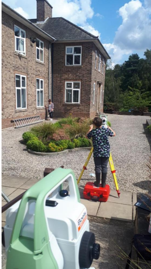
Photograph M_2: Volunteers learning to use EDM Total Stations to survey the exterior of Ransom Hall.
