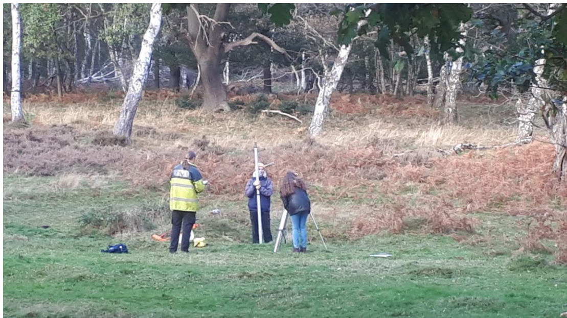
Photograph A_6 : Students from Nottingham University undertaking a 3D survey of a military pit, with an Auto Level (Dumpy Level) during a training session in Birklands Wood.
