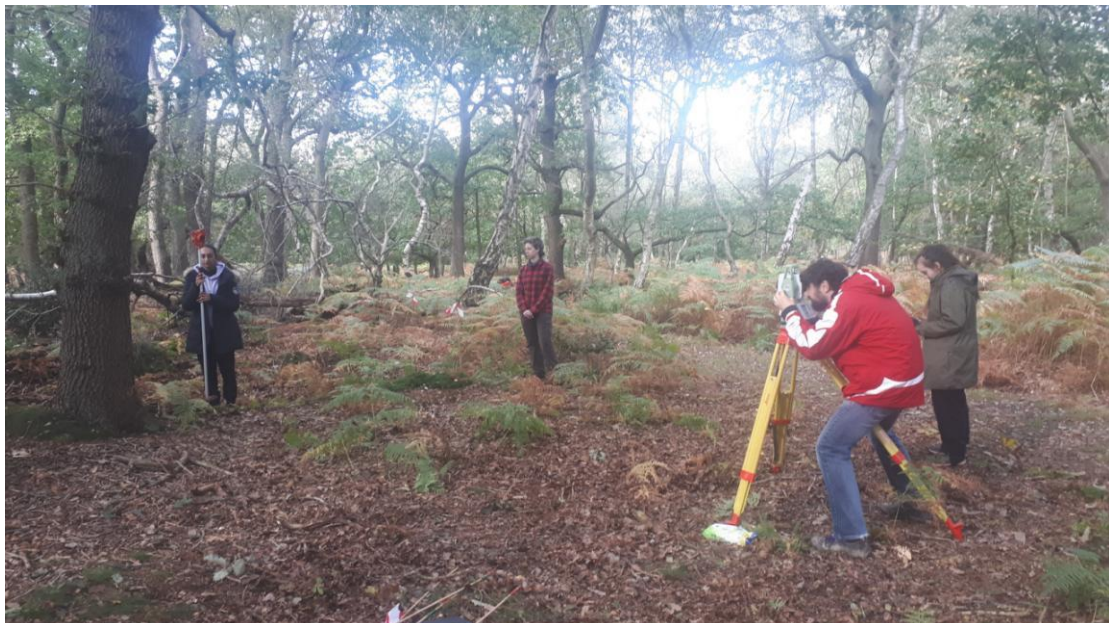
Photograph A_10 : Volunteers undertaking Level Two Survey using EDM Total Station in Birklands nnr (Sherwood Forest National Nature Reserve, 2021).
