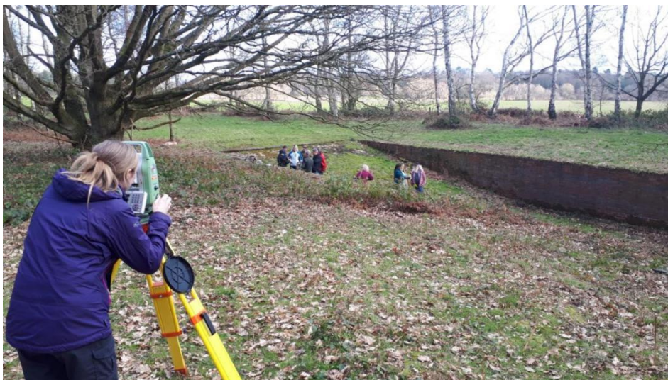
Photograph N_11: Volunteers undertaking Level Two survey with an EDM Total Station.
