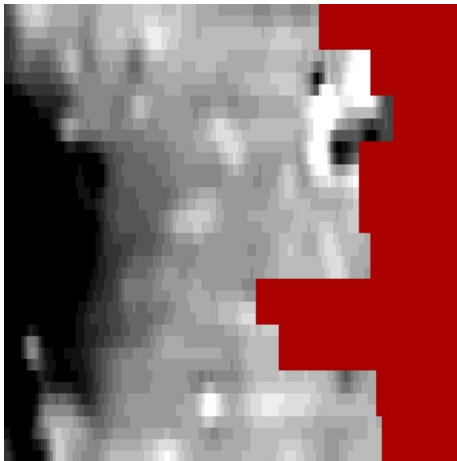
Figure 19: Magnetometer data greyscale image area 3, Clipped +4NT/ - 15NT, Destriped, De-Spiked (Threshold 1.0), Interpolated Vertical
