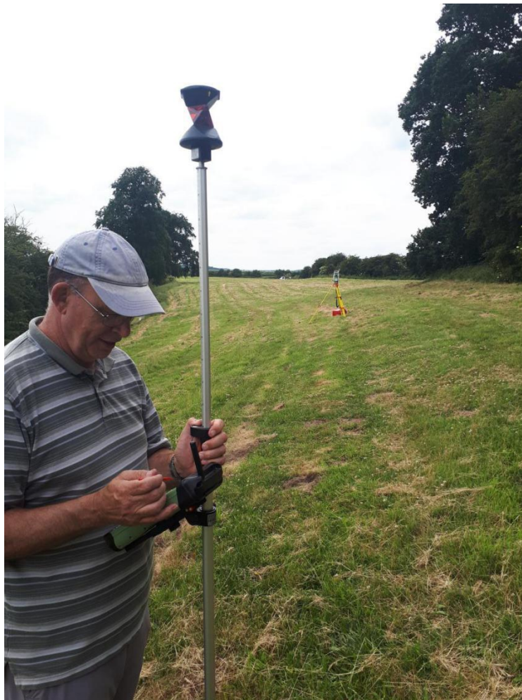
Photograph 1: Volunteer Kevin Williamson undertaking objective survey using a Leica Robotic Total Station.
