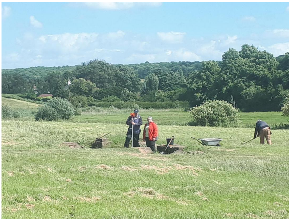
Photograph 2: Volunteers Bob and Sue Longden recording stone sluices using a Leica TS06 EDM Total Station.
